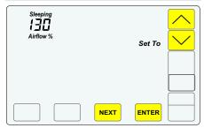
The Sleeping Airflow% is displayed. Press or to adjust the amount of heating or cooling to the upstairs sleeping zone. Press <u>ENTER</u> to save the new airflow setting. The upstairs temperature (Sleeping) is displayed and used to control heating and cooling calls.
