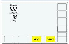
The Sleeping and Living Airflow% are displayed. Press ENTER to have the thermostat automatically adjusts the distribution of heating and cooling to the upstairs and downstairs zones to keep the spaces within 2 degrees of each other.
