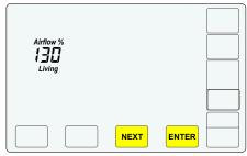
The Living Airflow% is displayed. Press or to adjust the amount of heating or cooling to the downstairs living zone. Press ENTER to save the new airflow setting. The downstairs temperature (Living) is displayed and used to control heating and cooling calls.
