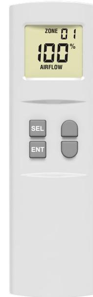
**The WRCD is typically used to control airflow to one space and defaults to Zone 01 and Address 01. If your installation has Zone and/or Address numbers different than the default, see page 2 for instructions on setting the Zone and/or Address number before adjusting the airflow. If the Zone and/or Address number is not set correctly for the space, the damper will not respond.**
